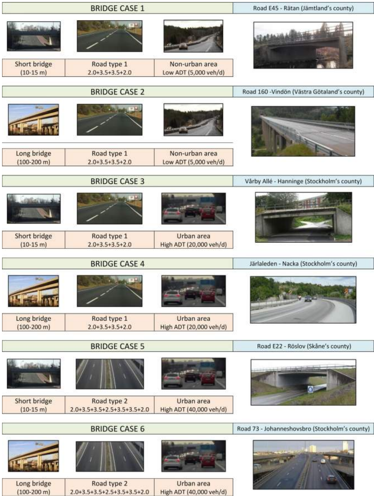
Figure 6. The six BCs accounted in the LCCA identified by the combination of the parameters and with an existing Swedish bridge example for each case.
